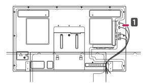
2 Mount the speaker by using a screw as shown in the following. Then connect the speaker cable.
